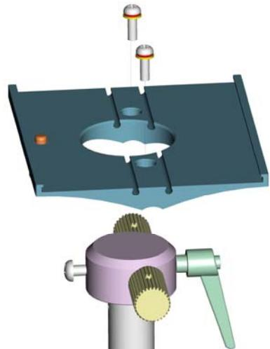
8 Level the handrail basket at the top two concave blocks and fix them with four H screws.
