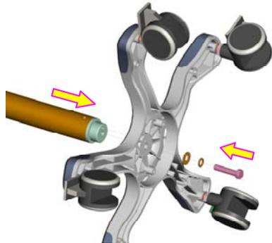
4 For MT-207 Trolley, a balancing weight is installed on the chassis. You should take it off first. After installing the stand post as shown in step3, fix the balancing weight back to chassis by using three screws.
