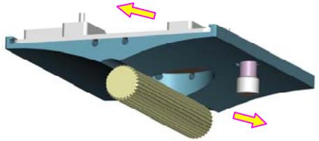
6 Loosen two screws on the top splint to take off the rotary axis, then pull the rotary axis through the flange hole of lifter rod. Insert the L-shape angle adjustment handle and a G screw into the two holes of flange, but do not tighten them.
